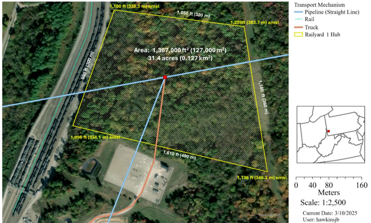
Figure 26. Land sat image of the Railyard 1 Hub Area. The yellow hashed area is the potential location for the hub. The elevations of the corners of the lot are shown in yellow text. The linear distance of the edges of the lot are shown in white text. The area of the lot is also shown.
