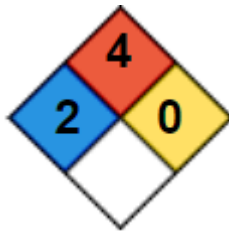
Compressed Natural Gas
