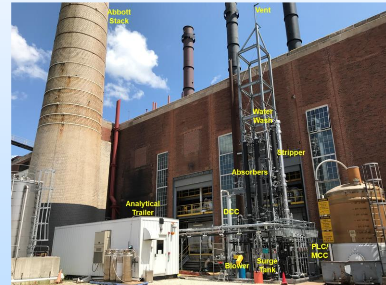
Small pilot-scale (40 kWe) skid of ISGS' Biphaseic CO 2 Absorption Technology installed at the University of Illinois' Abbott Power Plant
