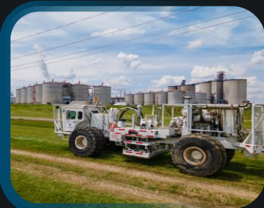
3D SEISMIC ACQUISITION
